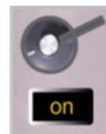
**The speed control.** Located at the bottom left of the record player, the speed control dial can be adjusted by clicking and rotating. The target speed can be set in the range between 0 and 90 rpm, and this speed is shown in the digital display in the bottom left corner.
