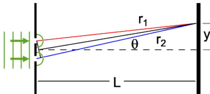
Figure 9: Monochromatic Laser Light Through Two Slits
