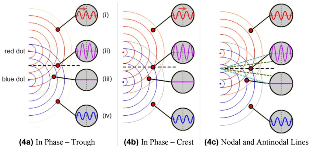
Figure 4: Interference of Two Overlapping Circular Waves
