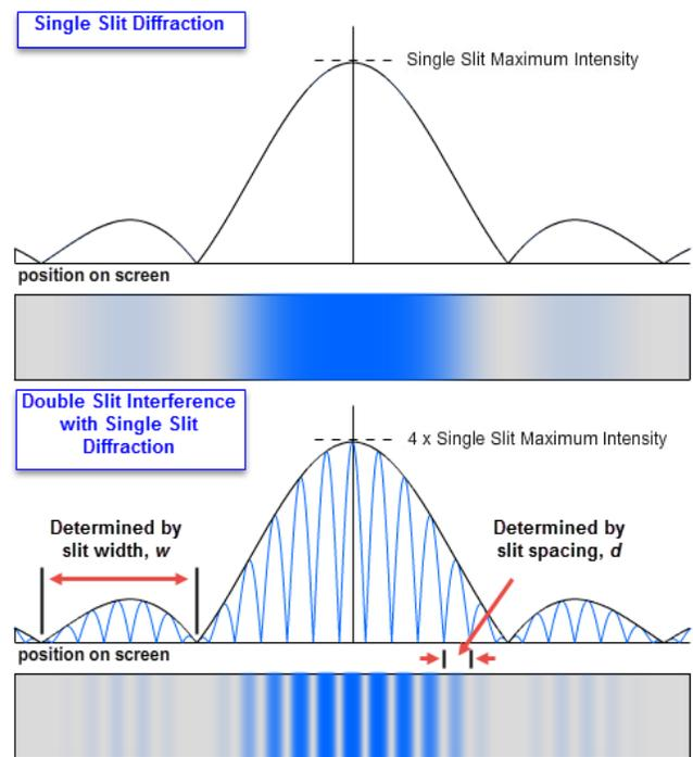
**Figure 21:** Double Slit Interference with Single Slit Diffraction
