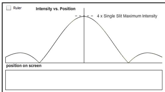
**Figure 14:** Double Slit Intensity and Fringe Pattern
