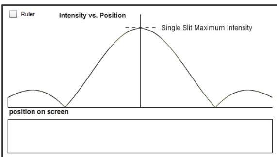
**Figure 15:** Single Slit Intensity and Fringe Pattern
