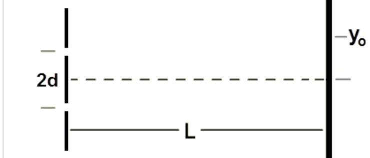
**Figure 12:** The Effect of Slit Spacing on the Location of Maxima
