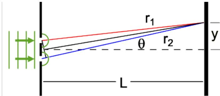
**Figure 11:** The Geometry of Interference Patterns
